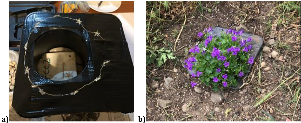
Figure A9. a) Sealed system prior to burial; b) PMFC system installed in the field with Campanula portenschlagiana .
