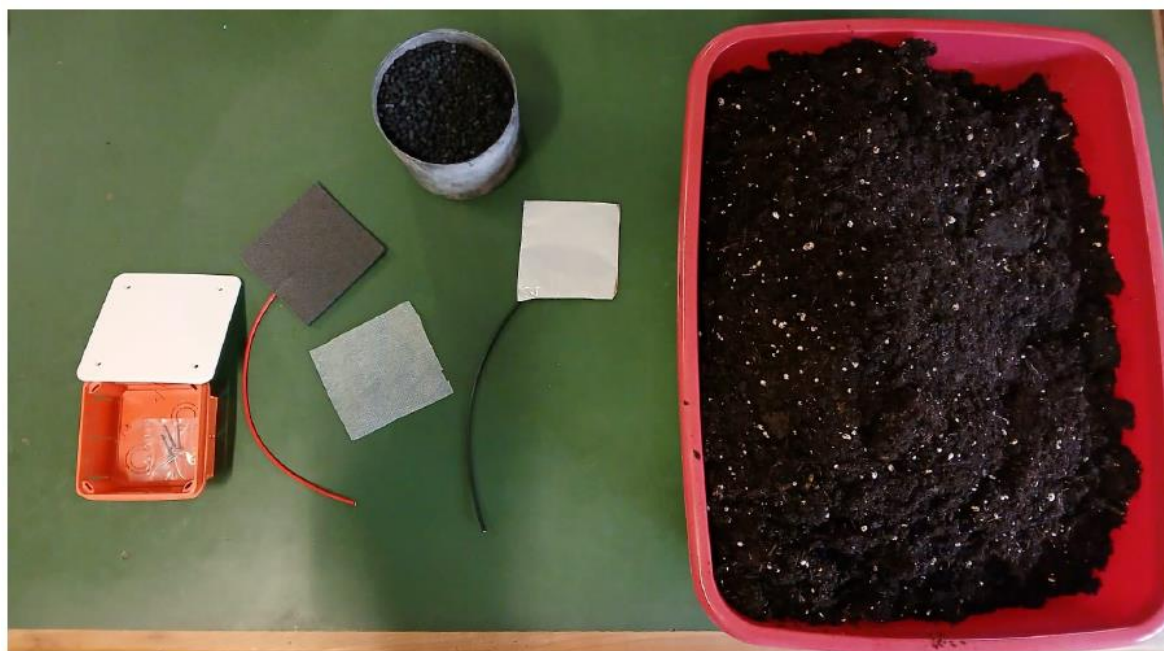
Figure 3.2. Cells components: derivation box, anode, non-woven fabric, carbon pellet, cathode and soil.
