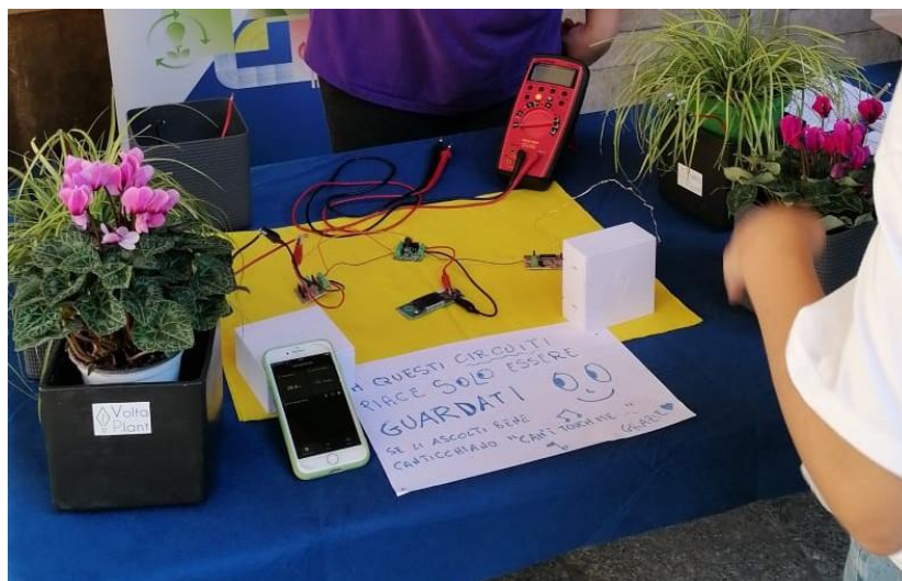
Figure A17. PMFC prototype powering LED lights and the environmental sensor simultaneously. The sensor is connected to the MyAmbience app, visible on the mobile screen.
