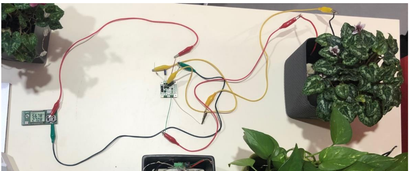
Figure A14. PMFC powering environmental sensor via the circuit system.
