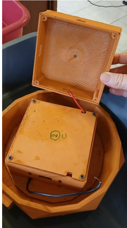
Figure A19. Compartment above the MFC, to be fitted with the electronic component.
