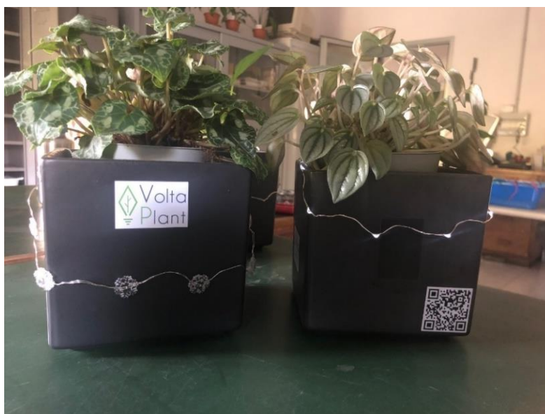
Figure A5. First demonstration prototype of PMFCs powering LED light strips.
