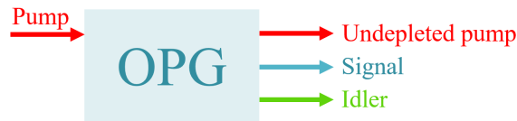
FIGURE 6.1: Schematic of optical parametric generation.
