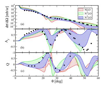
FIG. 10. Scattering observables as a function of the center-of-mass scattering angle  $\theta$  for elastic proton scattering on  $^{16}\text{O}$  computed at 200 MeV (laboratory energy) with the EGM potential [44] at different orders: red bands are the NLO results, green and blue bands are respectively the N<sup>2</sup>LO and N<sup>3</sup>LO results. Data are taken from Refs. [65,66].
