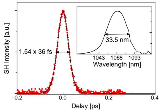
Fig. 4. Autocorrelation trace and corresponding optical spectrum (inset) of the shortest pulses obtained with Yb:CALGO.
