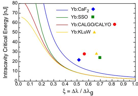
Fig. 3. Intracavity critical pulse energy calculated from our experimental conditions according to Eq. (5) (colored lines) and measured intracavity pulse energy as a function of  $\xi$  parameter at the start of the soliton ML regime (colored dots).
