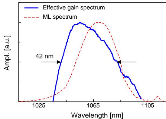
Fig. 2. Effective gain spectrum of Yb:CALGO calculated in our experimental conditions. The measured ML spectrum corresponding to the shortest pulses obtained is also shown in dashed red.
