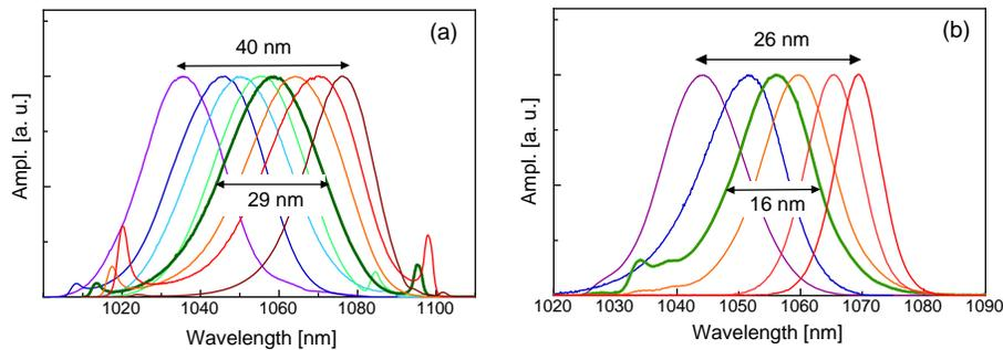
Fig. 5. Central output wavelength tuning range in single DP setup for Yb:CALGO (a) and Yb:KLuW (b).
