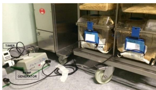
Figure 1. PEMF treatment setup. Pulsed electromagnetic field device (PEMF generator) connected to the coil fixed at the bottom of rat cages and controlled by a timer for 8h/day for 15 days.
