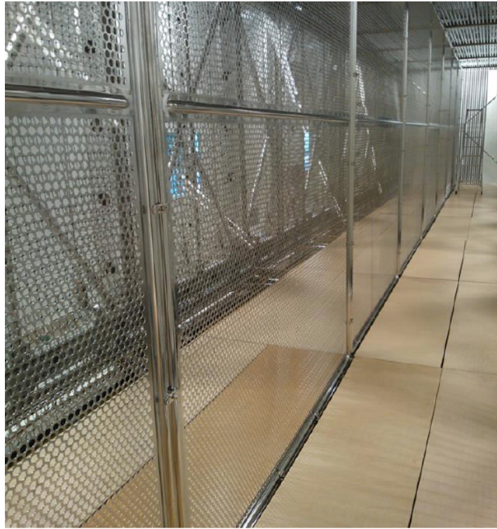
Figure 2.16: Cathode panels after flattening, cleaning and reinstallation for the first T300 module.
