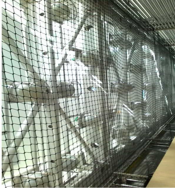
Figure 2.14: Picture of PMTs installed in the first T300 module.
