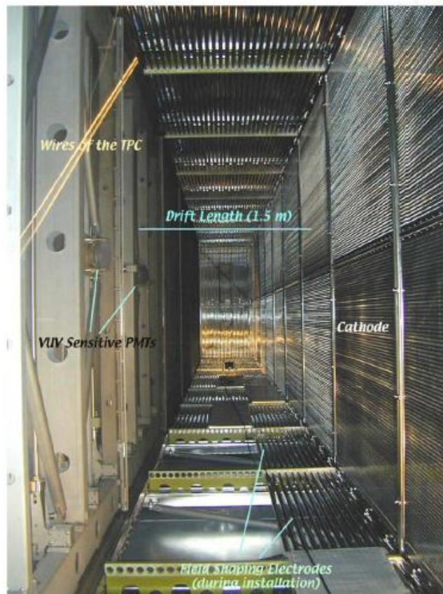
Figure 2.2: Picture of the inner detector layout inside the first half-module: the cathode (vertical plane on the right) divides the volume in two symmetric sectors (chambers). The picture refers to the left sector where wires and mechanical structure of the TPC and some PMTs are visible.
