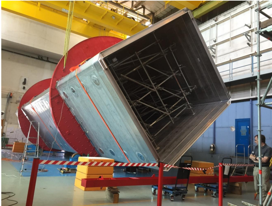
Figure 2.17: First cold vessel in the present stage of assembly at CERN. In this picture, the top part of the vessel, already completely assembled, lies on the bottom.
