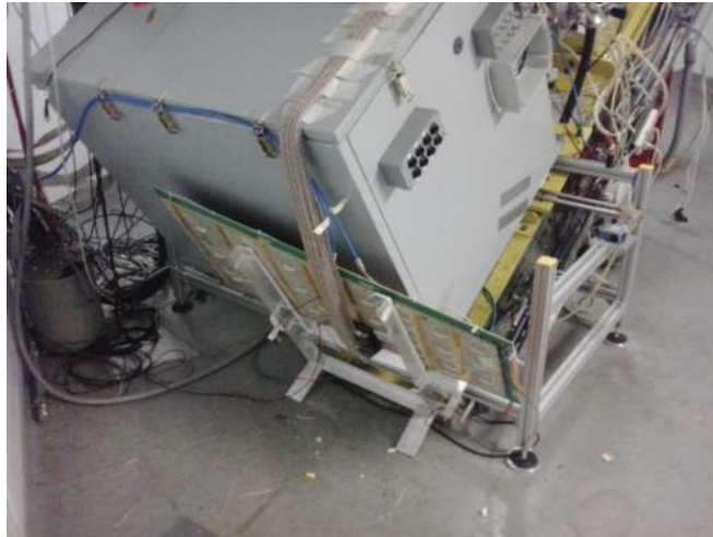
Figure 3.31: GE1/1-III Triple-GEM detector installed at the Louvain-la-Neuve facility.
