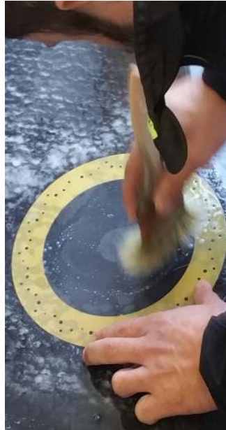
Figure 5.78: Cleaning of the FTM PCB foils: the foil is washed with water and an industrial soap, scrubbed with a brush and then rinsed.
