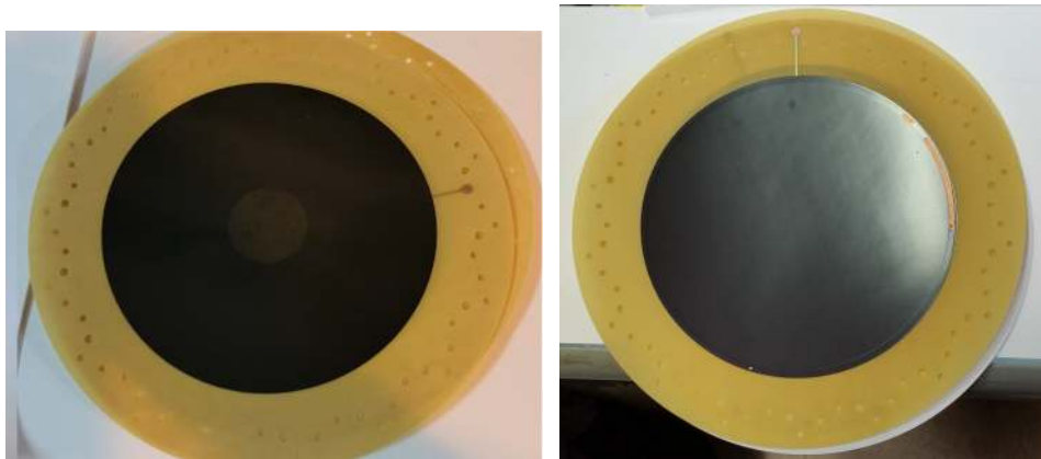
Figure 5.75: Pictures of PCB foils with holes (on the left) and full (on the right) taken during the assembly.
