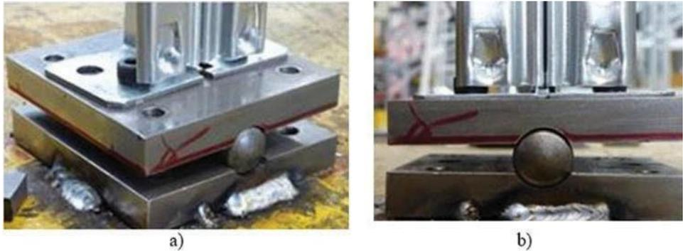
Figure 5-12. Details of the hinged base restraint.
