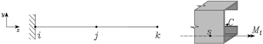
The torsional moment applied at the free end is  $\bar{M}_t = 0.01 \text{ kNm} = 10000 \text{ Nmm}$ . The boundary condition associated with the applied loads are:  $\bar{\varphi}_x(x) = 0$ ,  $\varphi_x(0) = 0$ ,  $\dot{\varphi}_x(0) = 0$ ,  $B(L) = 0$  and  $M_t(L) = 10000 \text{ Nm}$ . Main numerical values are reported in the following table.
