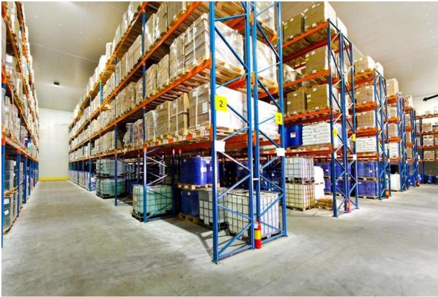
**Figure 1-1. Steel storage pallet racks.**
