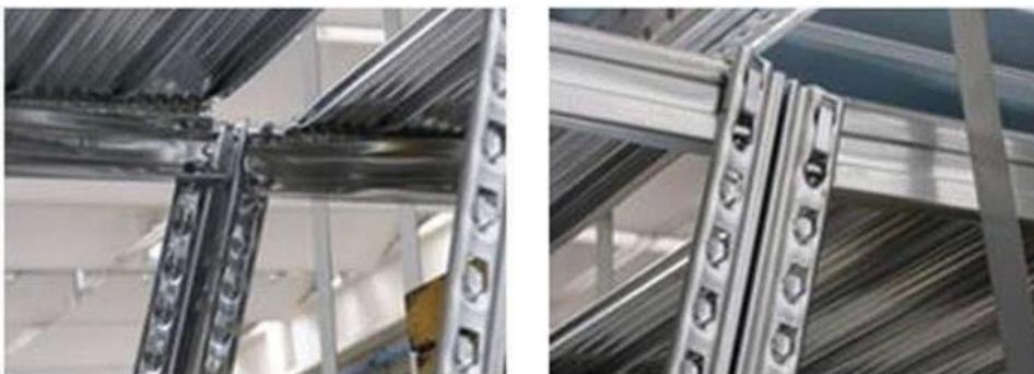
Figure 5-19. Details of the beam-to-column joints after tests.
