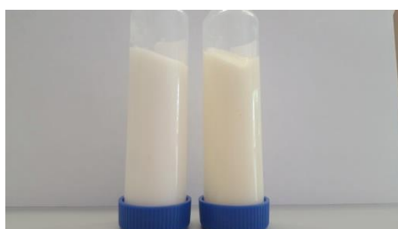
Figure5. Discoloration for F5 sample treated with UV-vis irradiation (on the left) respect to t0 sample (on the right).
