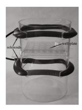
**Figure 3.4**: Electromagnetic bioreactor. Solenoids of the electromagnetic bioreactor with a culture well-plate in the central region [295]
