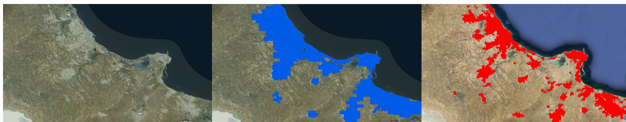
Figure 4.4: Urban maps for Sousse and Monastir, Tunisia; left:Google Earth TM , middle: CCI-LC 2010 urban map, right: result from the proposed map updating procedure.
