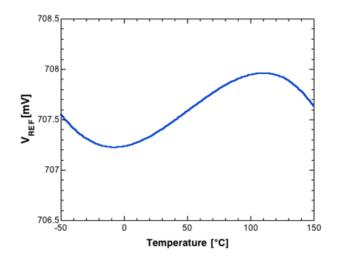
Figure 2.16: voltage at the output of the BGR based on bipolar devices simulated in nominal condition.
