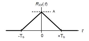
Figure 3.8: autocorrelation of a random NRZ stream.
