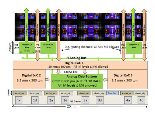
Figure 1.9: preliminary floorplan of the RD53A chip
