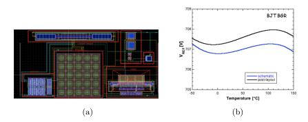
Figure 2.19: (a) proposed layout and (b) comparison between pre and post layout simulations of the bandgap reference with bipolars transistors.
