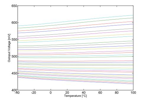
Figure 2.26: output voltage vs. temperature for the 32 possible values of  $R_0$ .
