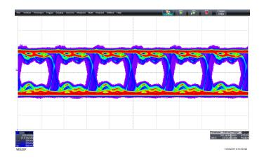
Figure 3.56: measured eye diagram of the receiver in nominal condition at 1.2 Gbit/s.
