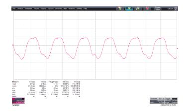
Figure 3.52: measurement of the differential output of the transmitter stimulated by a clock signal at 640 MHz.
