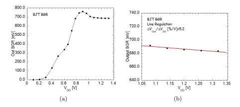
Figure 2.28: (a) output voltage of the bandgap vs power supply and (b) line regulation for the bandgap based on bipolar devices.
