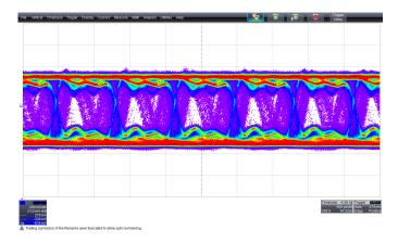
Figure 3.53: eye diagram of the receiver, as a response to a differential PRBS at 1.2 Gbit/s and differential input of  $V_{ID} = 100 \text{ mV}$  (worst case condition). The measurement has been performed at the output of the CML driver.
