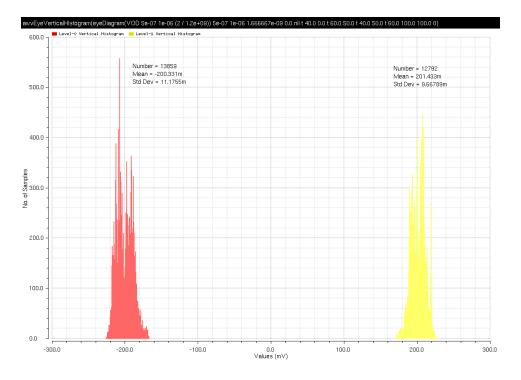
Figure 3.28: histogram of the eye diagram levels
