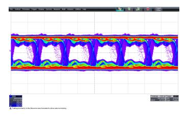
Figure 3.55: eye diagram receiver output, as a response to a PRBS at 1.2 Gbit/s and with  $V_{ID} = 150$  mV. This is the minimum detectable signal at 1.2 Gbit/s.
