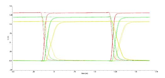
Figure 3.42: Eye diagram of the receiver output from PVT simulations. Red line refers to the fast corner, green line to the typical corner and yellow line to the slow corner.
