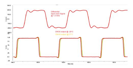
Figure 3.40: transient response of the receiver when a 1.2 GHz clock signal is applied for two operating temperatures: -20 °C (red line) and 27 °C (yellow line).
