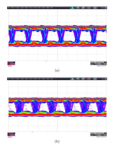
Figure 3.58: eye diagram measurements for the receiver, stimulated by a 640 Mbit/s PRBS signal (a) before irradiation and (b) after irradiation with a TID of 550 Mrad.
