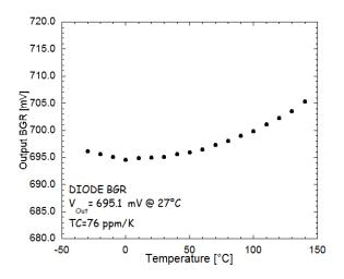
Figure 2.29: output voltage vs. temperature for the bandgap based on diode.
