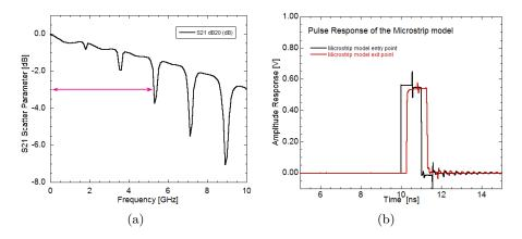
Figure 3.25: (a) S21 insertion loss scatter parameter of the microstrip and (b) impulse response of the microstrip line.
