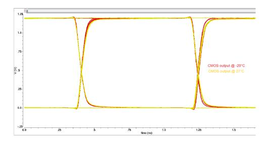
Figure 3.39: eye diagram of the output receiver signal. Stimulated by a PRBS signal 1.2 Gbit/s and differential input signal  $V_{ID} = \pm 200$  mV.
