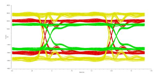
Figure 3.31: eye diagram simulated in three different corners: the green diagram obtained in the slow corner, the red one in the typical corner and the yellow one in the fast corner.
