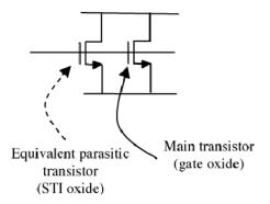
Figure 2.4: circuit model for an NMOS exposed to ionizing radiation with the parasitic devices due to charge trapped in the STI.
