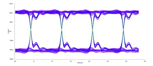
Figure 3.27: simulation of the transmitter eye diagram taken at the input termination resistance of the receiver.
