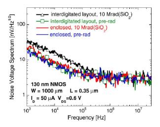
Figure 2.8: Noise voltage spectra before irradiation and after exposure to a 10 Mrad total dose for NMOSFETs with enclosed layout and with interdigitated layout, at 50  $\mu$ A.
