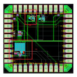
Figure 3.45: layout of the chip with transmitter and receiver (red box) submitted in May 2015.
