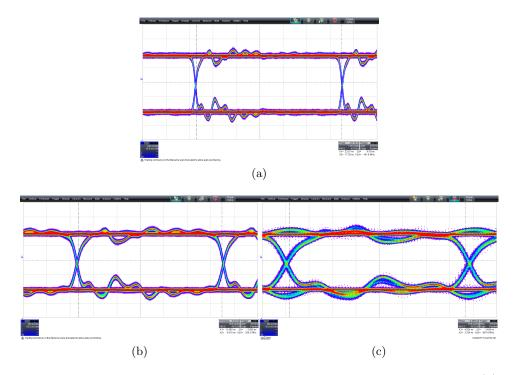
Figure 3.50: measurements of the eye diagram of the transmitter at (a) 160 Mbit/s, (b) 320 Mbit/s and (c) 640 Mbit/s.
