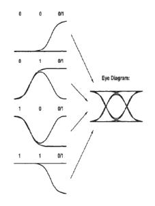
Figure 3.16: generation of the eye diagram.
