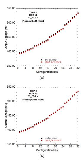
Figure 2.43: output voltage as a function of the configuration bits for two chips irradiated with a fluence of  $2 \cdot 10^{15}$  n.eq/cm<sup>2</sup> at the neutron source in Ljubljana.
