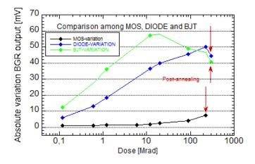
Figure 2.33: output voltage vs. TID for the three kinds of BGRs irradiated at room temperature and biased as in the real application.
