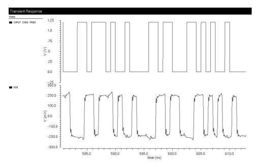
Figure 3.26: differential output of the transmitter. Stimulated with a PRBS at 1.2 Gbit/s.
