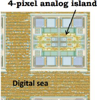
Figure 1.10: example of the new design approch. Four custom analog pixels are surrounded by a digital sea, where the digital standard cells are automatically placed and routed by synthesis tool.
