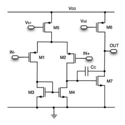
Figure 2.13: schematic of the proposed operational amplifier.
