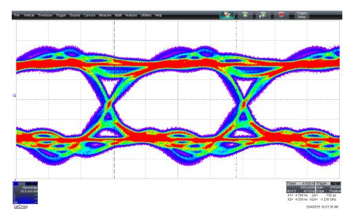
Figure 3.48: eye diagram at 1.2 Gbit/s of the transmitter signal.
