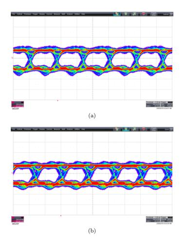
Figure 3.57: eye diagram measurements for the transmitter, stimulated by a 1.2 Gbit/s PRBS signal (a) before irradiation and (b) after irradiation with a TID of 550 Mrad.
