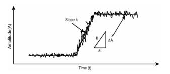
Figure 3.15: amplitude noise to timing jitter conversion through the linear model.
