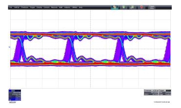
Figure 3.54: eye diagram of the receiver as a response to a differential PRBS at 640 Mbit/s and differential input of  $V_{ID} = 100$  mV. The measurement has been performed at the output of the CML driver.
