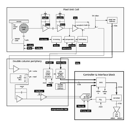
Figure 1.7: block diagram of the PSI46DIG ASIC chip.
