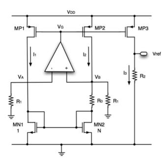
Figure 2.12: schematic of the current mode bandgap voltage reference based on MOSFETs in sub-threshold region.
