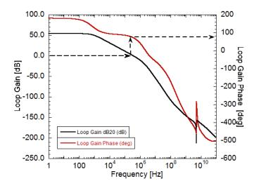
Figure 3.20: Bode diagram of the common mode loop gain.
