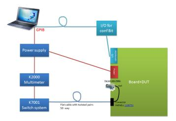
Figure 2.35: block diagram of the automated test system.
