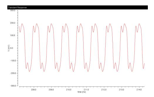
Figure 3.30: differential signal at the driver output. Input signal is a clock at 1.2 GHz at room temperature and nominal condition.
