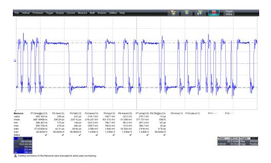
Figure 3.49: measurement of the output waveform of the transmitter, with the relevant parameters.
