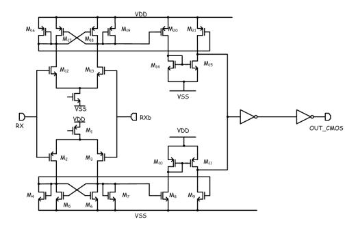
Figure 3.34: schematic of the receiver.
