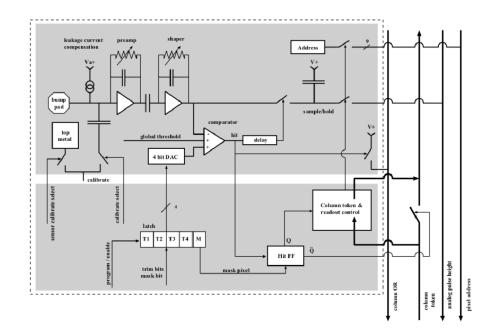
Figure 1.5: block diagram of the pixel cell of the PSI46V2 chip employed in the CMS innermost silicon pixel layer.
