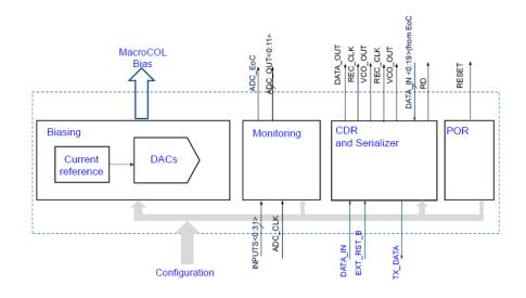
Figure 1.15: analog chip bottom block diagram.
