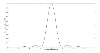
Figure 3.9: power spectral density of a random bit stream.
