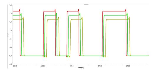
Figure 3.41: CMOS output of the receiver from PVT simulations. Red line refers to the fast corner, green line to the typical corner and yellow line to the slow corner.
