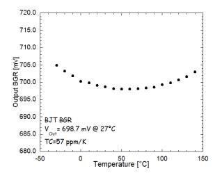
Figure 2.27: measurement of the output voltage vs. temperature for the bandgap based on bipolar transistors.
