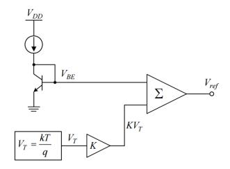
Figure 2.10: block diagram of the bandgap voltage reference.
