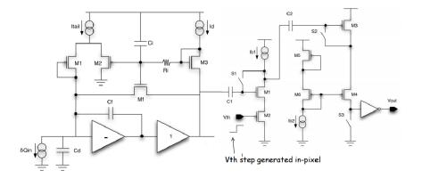
Figure 1.12: schematic of the analog pixel front-end designed at FNAL.
