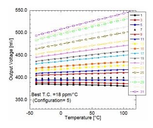
Figure 2.36: bandgap output voltage vs. temperature for different configurations of the trimming resistor.
