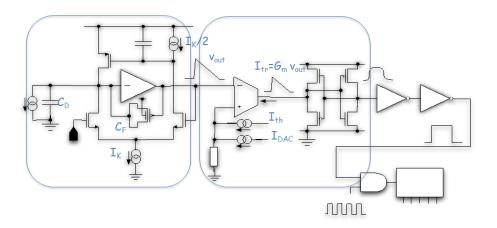
Figure 1.13: schematic of the analog pixel front-end designed at Universities of Bergamo and Pavia and INFN Pavia.
