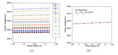
Figure 2.39: (a) output voltage vs. power supply and (b) line regulation for the second version of the bandgap based on MOS in sub-threshold region.
