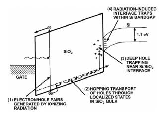
Figure 2.1: schematic energy band diagram for MOS structure, indicating major physical processes underlying radiation response.
