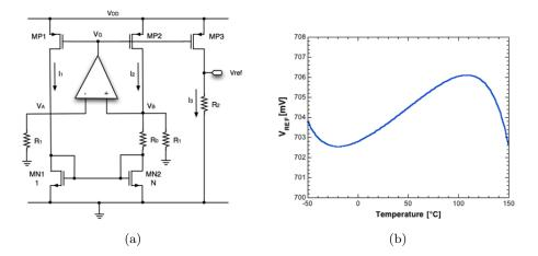
Figure 2.23: (a) schematic of the bandgap based on MOS in sub-threshold region and (b) output voltage as a function of the temperature in nominal conditions.
