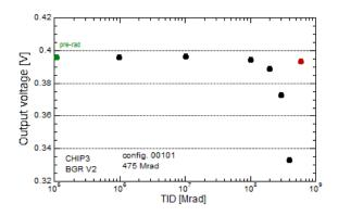
Figure 2.40: output voltage as a function of the dose in the sample irradiated with 10 keV X-rays.
