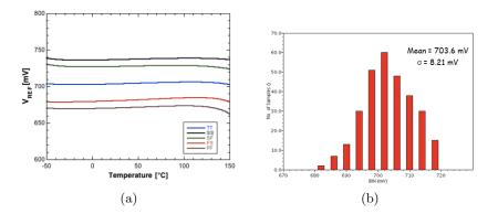
Figure 2.24: (a) output voltage for four corners simulations and (b) Monte Carlo simulations for the bandgap output voltage at room temperature.
