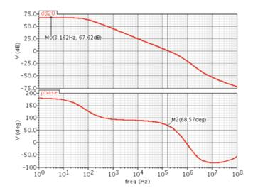
Figure 2.14: open-loop frequency response of the operational amplifier at room temperature.
