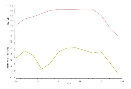
Figure 3.35: bandwidth and gain of the receiver as a function of the common mode voltage of the input signal.
