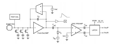
Figure 1.14: schematic of the analog pixel front-end designed at INFN Torino.
