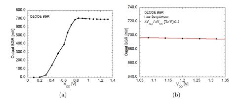
Figure 2.30: (a) output voltage as a function of the power supply and (b) line regulation of the bandgap based on diode devices.
