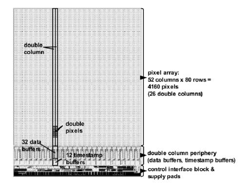
Figure 1.4: layout of the PSI46V2 chip employed in the CMS silicon tracker.
