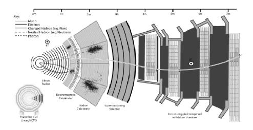
Figure 1.3: transverse section of the CMS detector and signatures for different particles crossing the volume.
