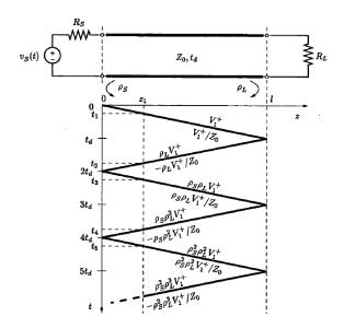
Figure 3.12: lattice diagram for a lossless transmission line with unmatched terminations.
