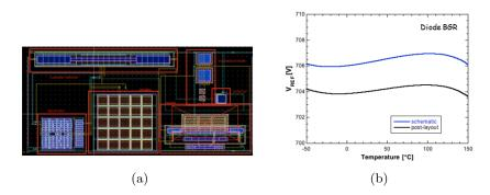
Figure 2.22: (a) layout and (b) comparison between pre and post layout simulations for the bandgap with diodes.
