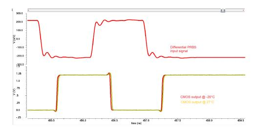
Figure 3.37: top plot is the PRBS differential input of the receiver at 1.2 Gbit/s and peak value  $V_{ID} = \pm 200$  mV. The bottom plot is the transient response of the receiver in nominal conditions for two different temperatures, -20 °C (red line) and 27 °C (yellow line).
