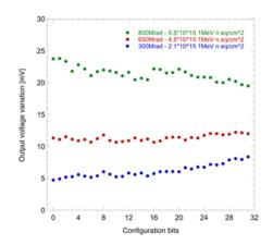
Figure 2.42: bandgap output voltage variation as a function of the configuration bits for different fluences and TIDs, from the 10 MeV proton source at the TANDEM accelerator in Legnaro.
