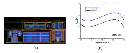
Figure 2.25: (a) layout and (b) comparison between pre and post layout simulations for the bandgap based on MOS devices
