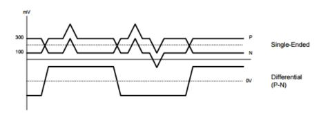
Figure 3.4: common-mode noise rejection.
