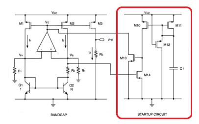
Figure 2.15: schematic of the proposed startup circuit.
