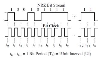
Figure 3.7: example of an NRZ random signal.
