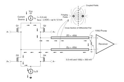
Figure 3.1: point-to-point LVDS link.
