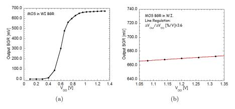
Figure 2.32: (a) output voltage vs power supply and (b) line regulation for the bandgap based on MOS transistors.
