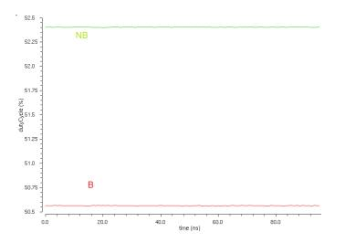
Figure 3.22: duty-cycle distortion during a transient simulation. The input signal is a clock at 1.2 GHz.
