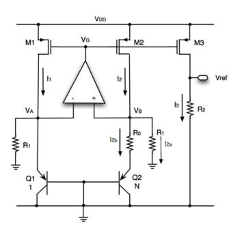
Figure 2.11: schematic of the current mode bandgap voltage reference based on bipolar devices.
