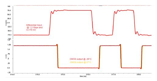
Figure 3.38: output CMOS of the receiver in worst case operating conditions  $(V_{ID} = \pm 70 \text{ mV}).$
