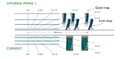
Figure 1.6: comparison between the current 3 layers (bottom) and the *Phase 1 upgrde* 4 layers for the CMS silicon tracker.
