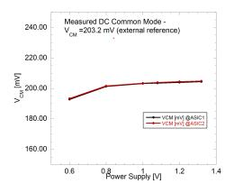
Figure 3.51: measured output common mode voltage  $(V_{CM})$  as a function of the power supply  $(V_{DD})$ .
