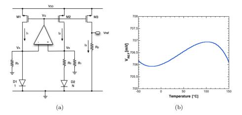
Figure 2.20: (a) schematic and (b) output voltage as a function of the temperature in nominal conditions for the bandgap reference circuit based on diode devices.
