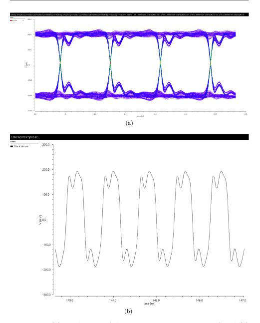
Figure 3.29: (a) eye diagram of the transmitter output at -20 °C and (b) transient response applying a clock input signal at -20 °C.
