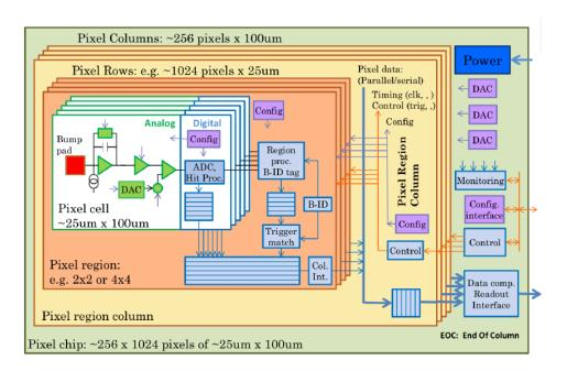
Figure 1.8: block diagram of the  $3^{rd}$  generation of front-end chip for the innermost layer of the CMS silicon tracker.
