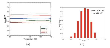
Figure 2.21: (a) output voltage as a function of the temperature as obtained from four corners simulations and (b) Monte Carlo simulation results for the bandgap based on diodes.
