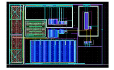
Figure 3.44: layout of the SLVS receiver.
