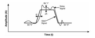
Figure 3.13: ideal digital signal and a noisy version of the same signal.
