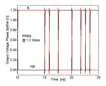
Figure 3.21: outputs of the Phase Splitter block, when at the input a PRBS signal at 1.2 Gbit/s is applied.
