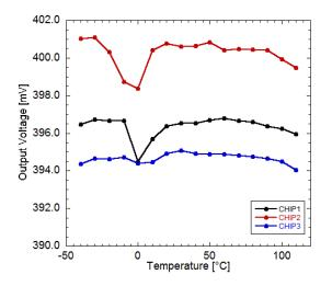
Figure 2.38: bandgap output voltage as a function of the temperature for three different chips.
