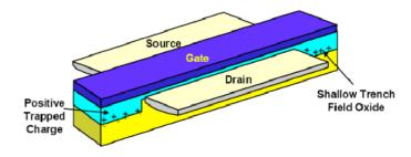
Figure 2.3: conceptual drawing (not to scale) showing how positive charge build-up in STI oxides can lead to lateral leakage currents in NMOS devices.
