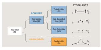
Figure 3.14: main components of the jitter: noise, system-phenomena and data-dependent contributions.
