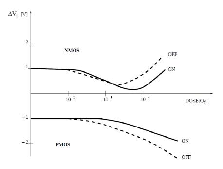
Figure 2.2: variation of the threshold voltage as a function of the Total Ionizing Dose (TID) for PMOS and NMOS devices.
