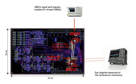
Figure 3.46: block diagram of the test bench setup and PCB test board with two ASICs, which are directly bonded on the PCB.
