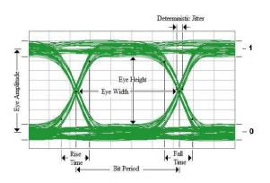
Figure 3.17: example of eye diagram with the relevant eye parameters.
