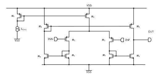
Figure 3.19: schematic of the symmetrical operational amplifier
