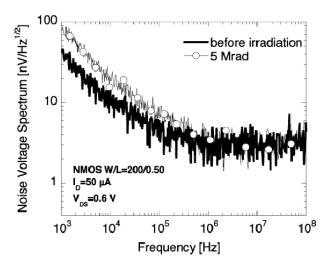
Figure 2.5: Noise voltage spectra before irradiation and after exposure to a 5 Mrad total dose of X-rays for an NMOS with W/L=200/0.5 in the 65 nm process, at 50  $\mu$ A drain current.
