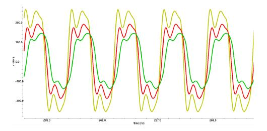
Figure 3.32: differential output of the driver, stimulated by a clock signal obtained from PVT simulations. The green time diagram refers to the slow corner, the red diagram to the typical corner and the yellow one to the fast corner.
