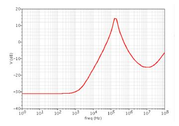
Figure 2.17: simulated PSR for the bandgap reference circuit based on bipolar devices.
