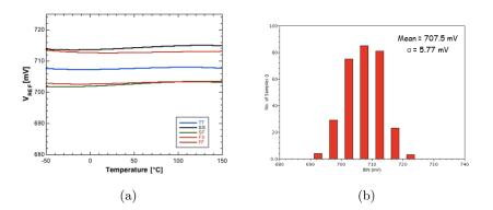
Figure 2.18: (a) four corners simulations and (b) Monte Carlo simulation for the bandgap reference circuit based on bipolar devices.
