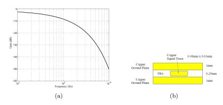
Figure 3.5: (a) S21 parameter and (b) cross-sectional view of 50 cm (FR4) PCB stripline.
