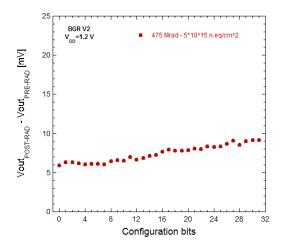
Figure 2.41: variation of bandgap output voltage after irradiation with 3 MeV protons at the CN accelerator in Legnaro.
