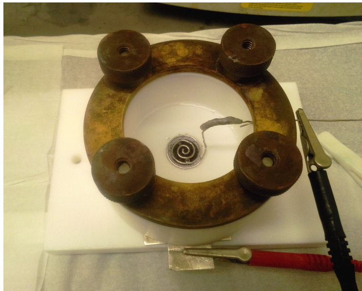
Figure 3.1: Photo of the assembled etch cell. The cell is made of Teflon and is secured with stainless steel cylinder and screws. The silicon wafer is visible from the hole in the bottom of the cell, fully covered by the HF solution. Just above the wafer, sealed with an O-ring, the platinum spiral-shaped cathode is also covered by acid solution, and is connected to the black wire that provides negative voltage. The anode is the silicon wafer, that is placed above an aluminum plate to which positive voltage is applied by the red wire. The wafer and the cathode are then fully covered by the HF solution.
