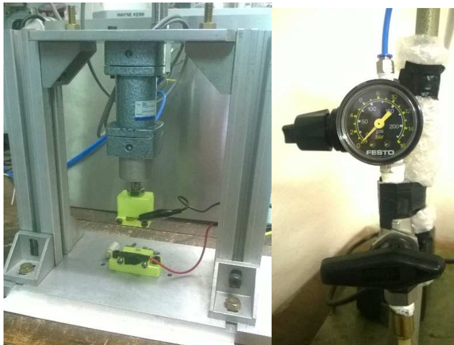
Fig. 3.3 Left: measuring instrument structure (with EAP test cell mounted on); Right: pressure reducer between compressor and piston.
