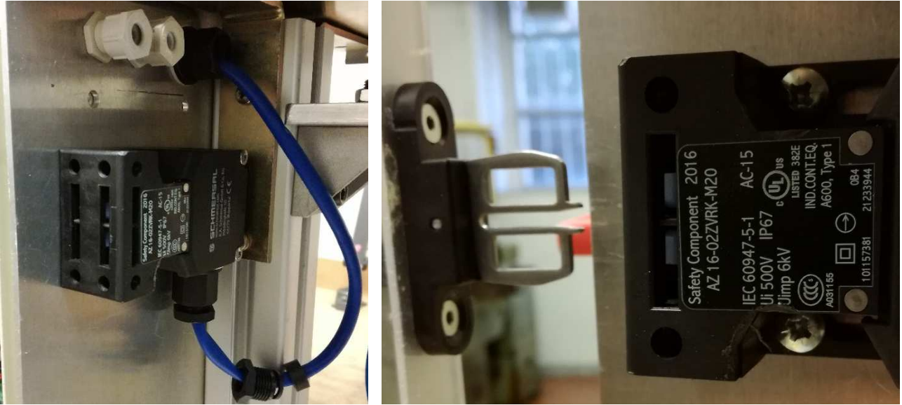
Fig. 3.10 Left: door microswitch mounted on the instrument structure; right: door key approaching to the structure microswitch.
