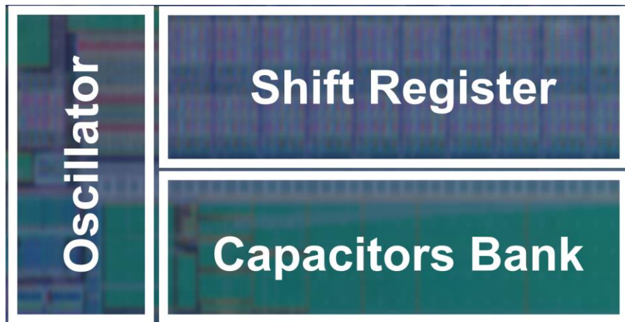
Figure 2.3: Silicon prototype (28nm) core photograph.
