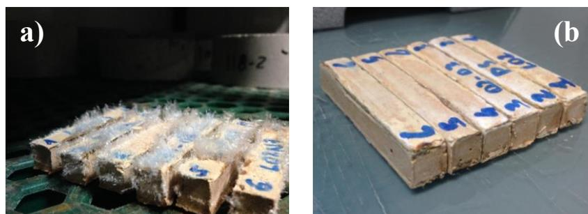
FIGURE 5.3. L02-100-8M\_1D binder (a) and L02-90-sPS-8M\_1D binder (b) after curing at 85°C for 20h. After curing the sample have been stored in a chamber at 25°C and at 99% R.H.
