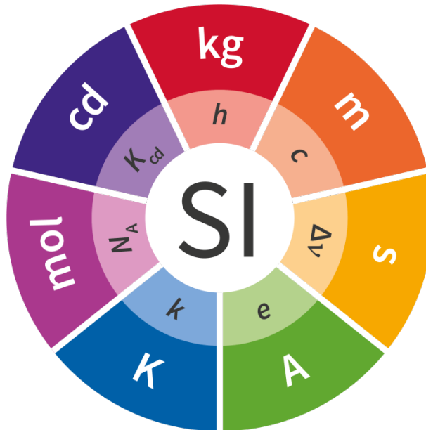
Figure 1: Illustration of 7 base units of SI with (in clearer version of the same color) the corresponding constant on which each definition will be based. [6]
