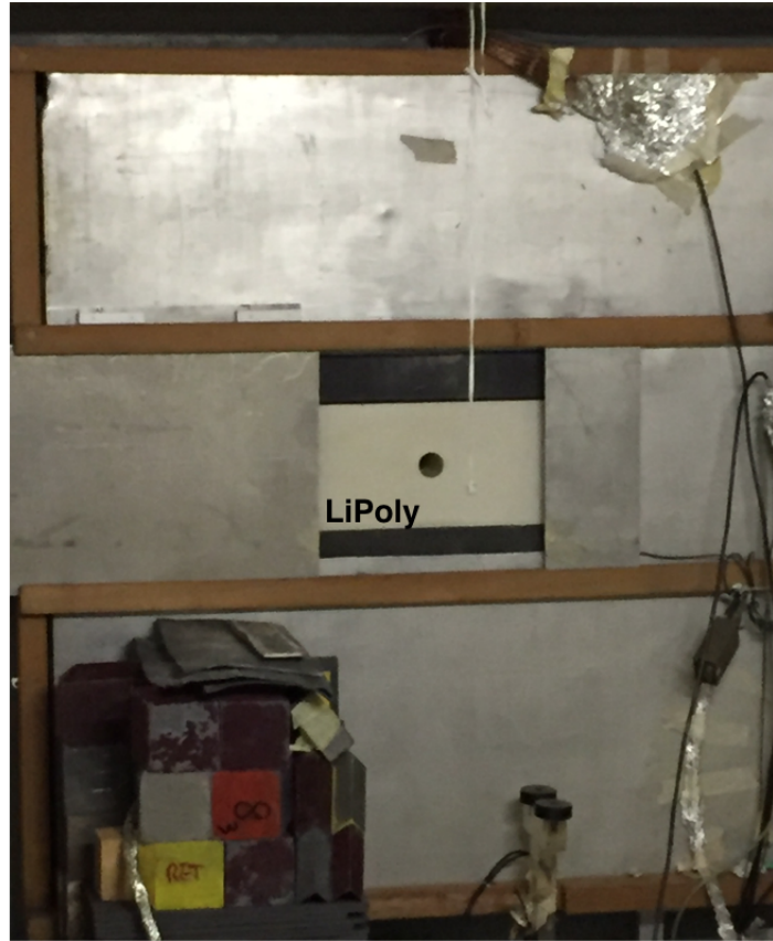
Figure 5.9: Irradiation chamber modification using 30 cm of natural Lithium Polyethylene with a 4 cm diameter neutron beam.
