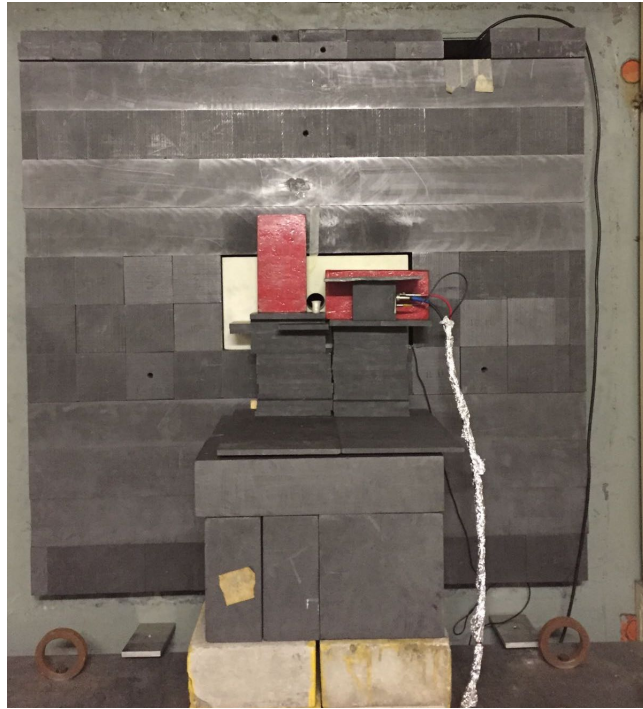
Figure 5.14: CZT prototype detector setup in the thermal column room without Boral shielding, the detector base is made of reactor grade graphite and the two red bricks are lead.
