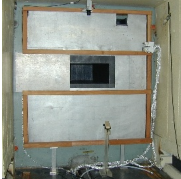
Figure 5.3: Image of the L.E.N.A. thermal column room with details of the 20 \times 40 \text{ cm}^2 irradiation chamber and the Boral shield with its sliding window.
