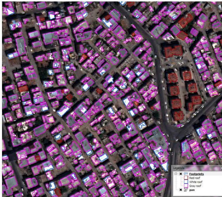
Figure 2.28: Results over a high density area in Izmir, Turkey. Buildings are separated by roof colour.
