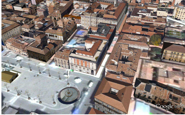
Figure 4.27: Example of 3D model used to estimate number of floors and material. Google ©.
