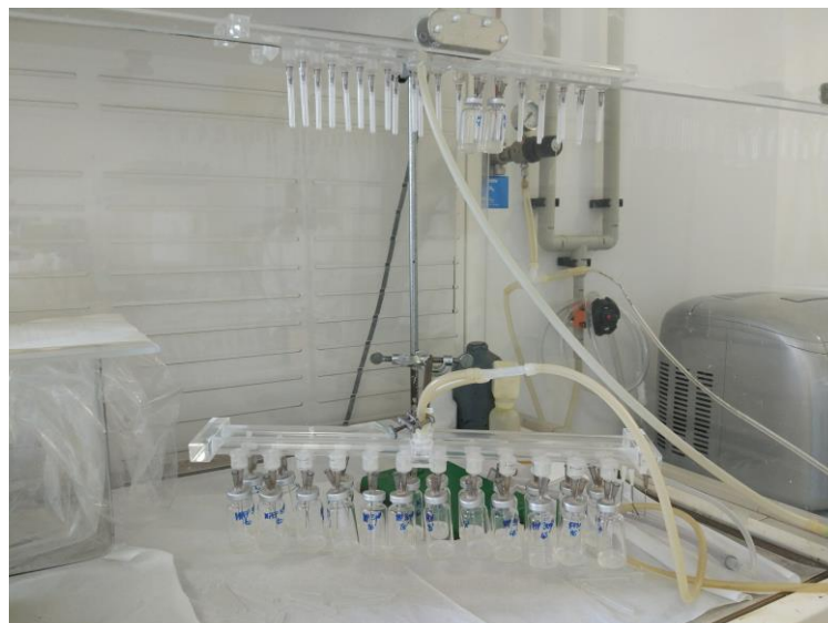
Figure 3.3. N 2 insufflation into sealed vials to make cells anoxic.
