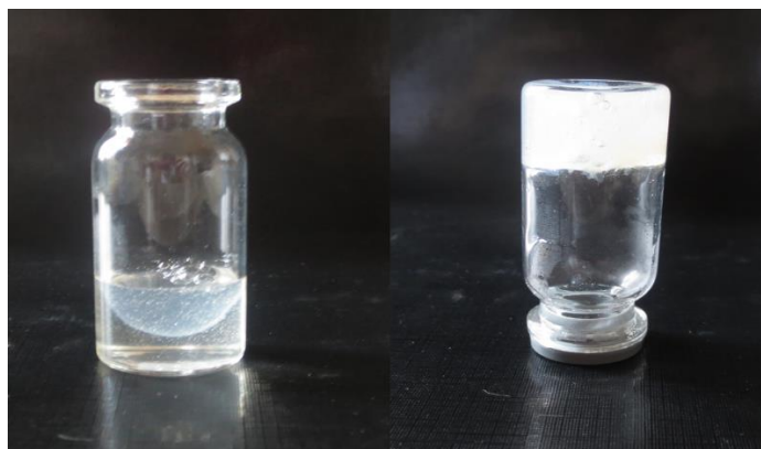
Figure S5. Photographs of chitosan solution added to alginate solution (left) and gel instantaneously formed after stirring (right).
