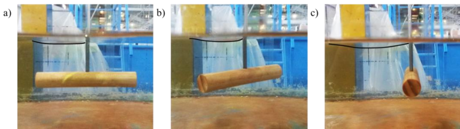
Figure 4.9 Photographs of configuration (a). a) Cylinder parallel to the flow; b) cylinder oblique to the flow; c) cylinder perpendicular to the flow. Black thick line follows the wave lower profile. Water flows from the right.
