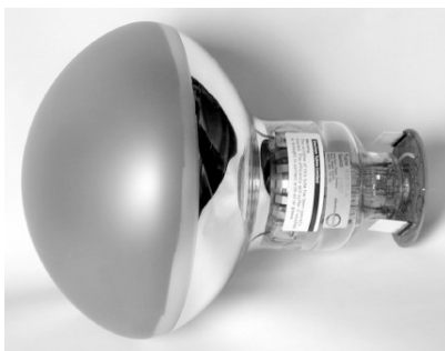
Figure 2.13: Picture of a Hamamatsu R5912-MOD photomultiplier.
