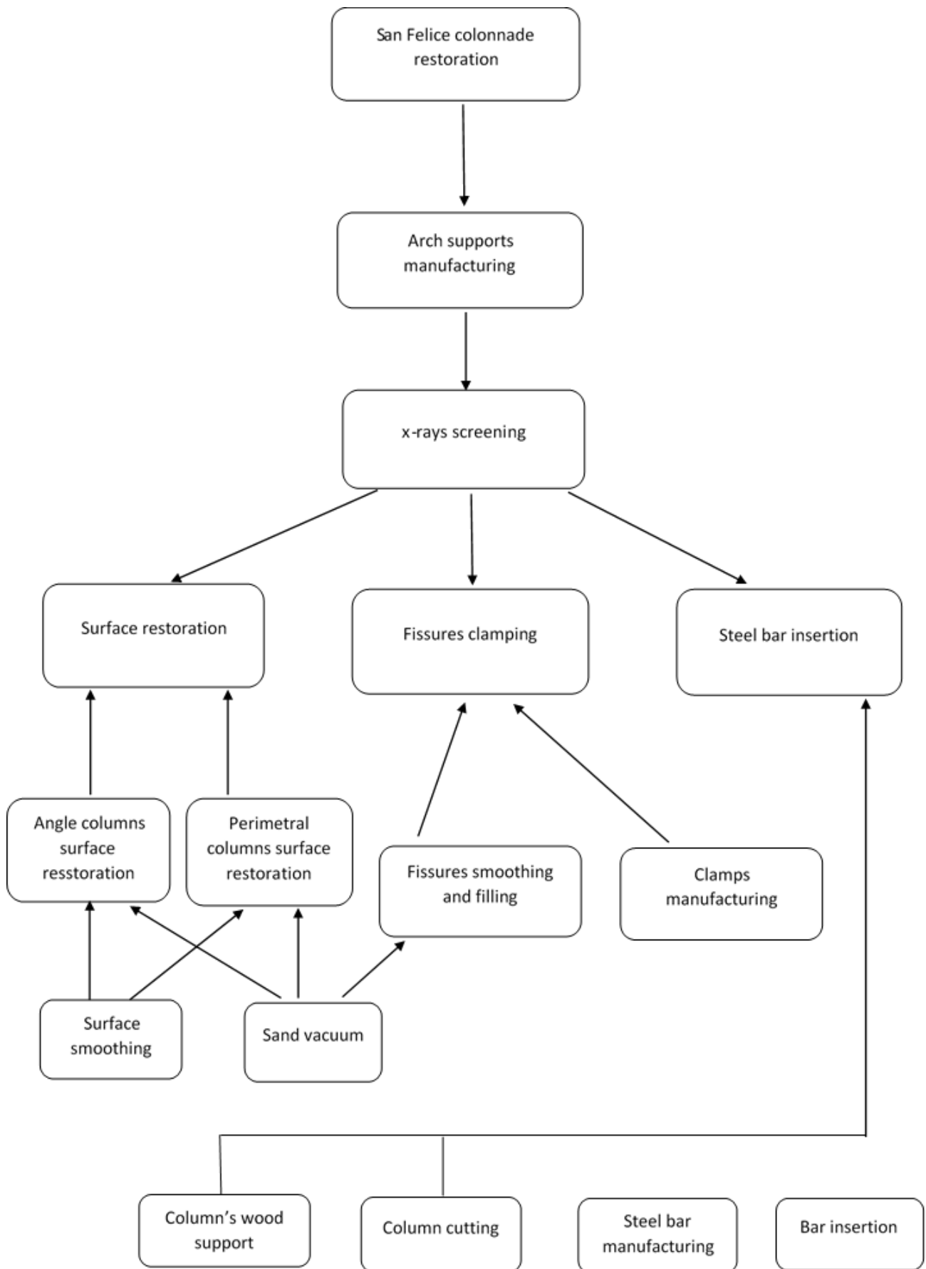
Figure 9. San Felice colonnade restoration's flowchart.
