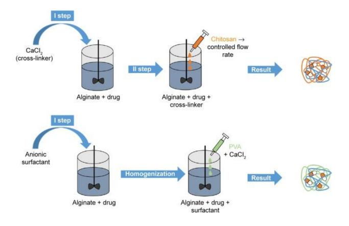
Figure 9. Production of hydrogel nanospheres, based on natural polymers.
