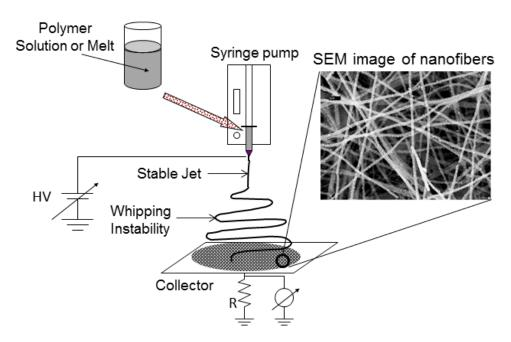
Figure 16. System for the production of the nanodevice.
