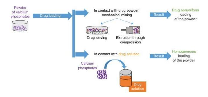
Figure 6. Processes exploiting the use of calcium phosphates involve mechanical mixing or contact between the powder and contact between the powder and drug solution, which leads to a homogeneous drug loading different from the mechanical mixing
