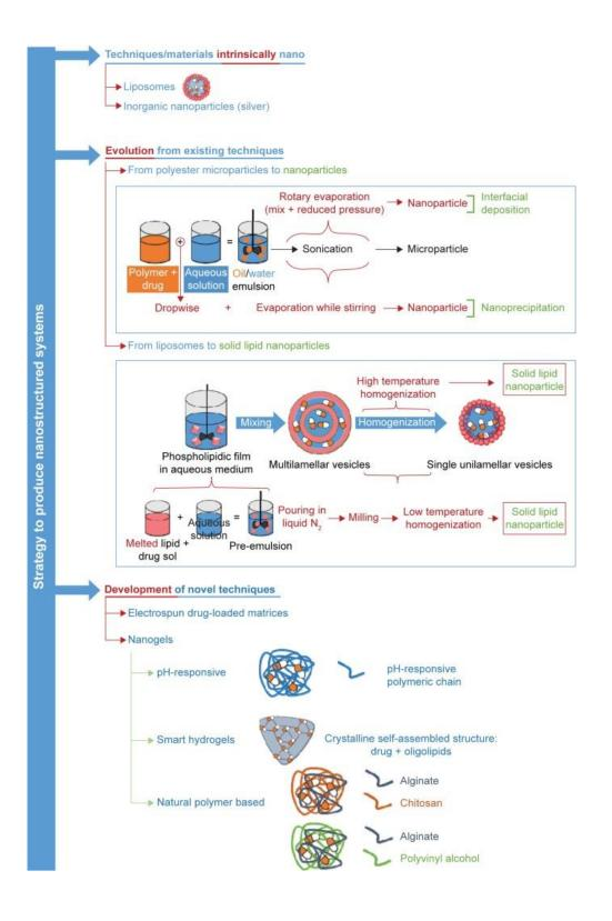
Figure 7. Scheme of nanostructured device production.
