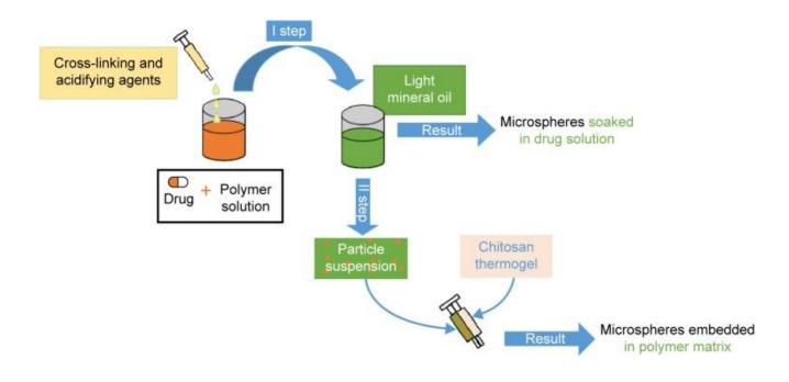
Figure 5. Fabrication process from thermoresponsive materials starts from a polymer–drug solution poured into light mineral oil to create a suspension of microspheres that can be mixed with another thermogel matrix to embed them in it.
