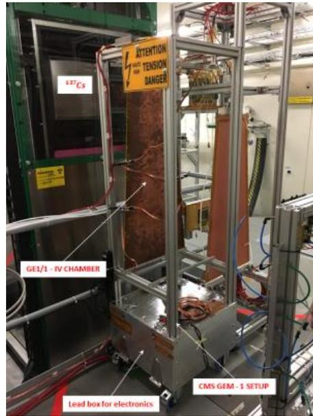
Figure 6.21: Picture of the longevity test at GIF++ facility. The GE1/1 triple-GEM detector is placed directly in front of the  $^{137}\text{Cs}$  source irradiator. The DAQ electronics is placed below the detector structure and is protected inside the lead shielding box. The entire system is connected to the DAQ station via USB cables.
