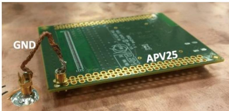
Figure 5.64: Close view of an APV25 Front-End ASICs plugged on the detector.
