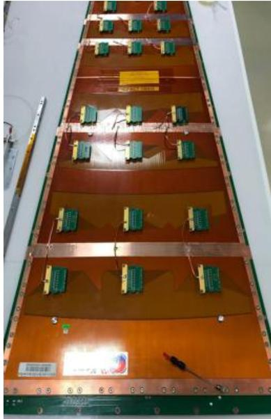
Figure 6.34: The detector under test is a triple-GEM detector equipped with korean GEM-foils based on the double-mask photolithography technique produced by the Mecaro company and operated in  $Ar/CO_2$  (70/30) gas mixture at an initial gas gain of  $2 \times 10^4$ .
