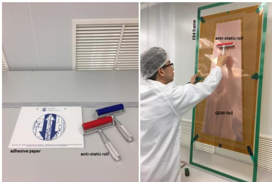
Figure 5.40: Cleaning of the GEM-foil with an anti-static roll in order to remove any possible dust particle deposited on the foil.
