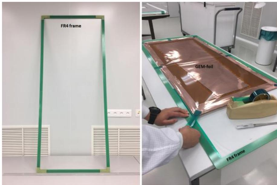
Figure 5.39: Preparation of the GEM-foil and installation on the FR4 frame.
