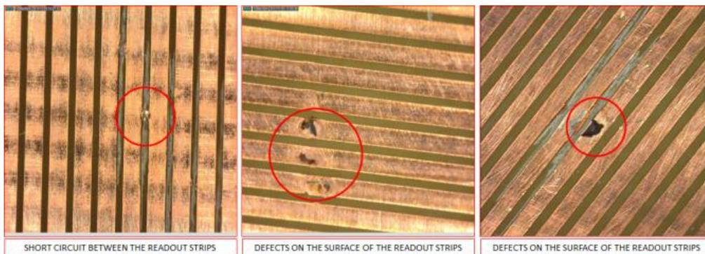
Figure 5.37: Microscopy photos of the readout strips showing some examples of defects and short circuits between the readout strips.
