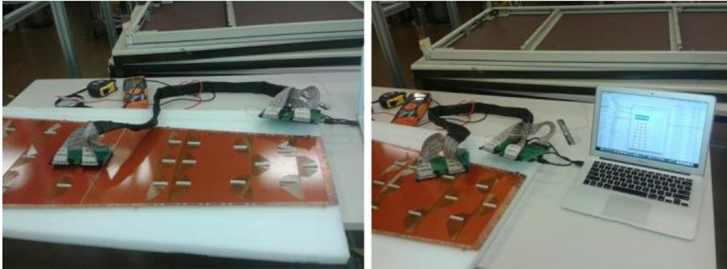
Figure 5.36: Pictures of the QC1 connectivity test setup.
