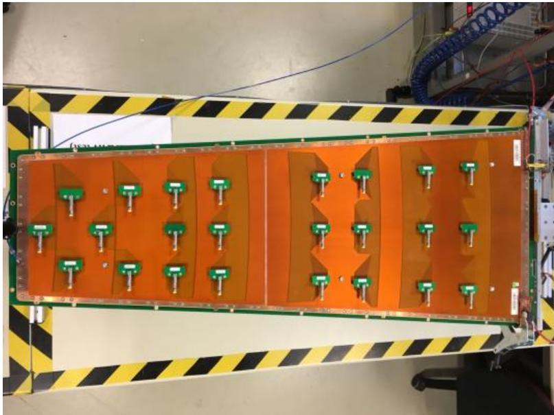
Figure 5.59: QC4 HV test overview of the detector with the Panasonic-to-LEMO and the 50 $\Omega$  terminations.
