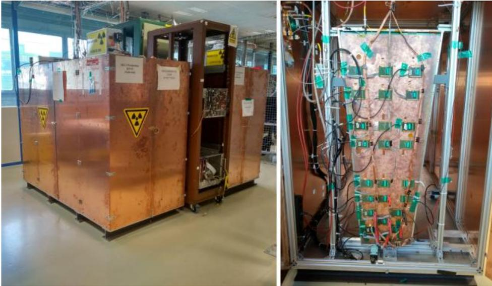
Figure 5.72: Picture of the experimental setup for the QC5 response uniformity test showing the X-ray generator, the DAQ stations (left) and the inside of the copper box with the electronics in place on the GE1/1 detector (right).
