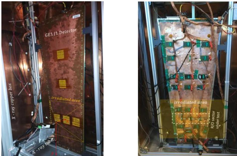
(a) The X-ray generator in front of the detector under test. (b) The detector under test equipped with the readout electronics.
