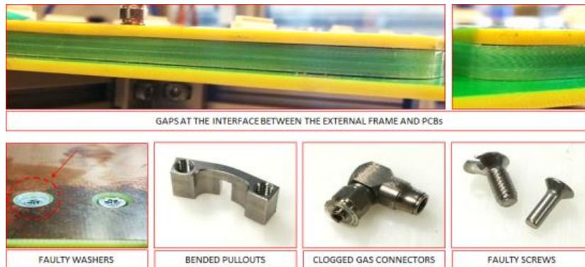
Figure 5.57: Examples of damage assembly components identified as potential gas leak sources in the GE1/1 detectors.
