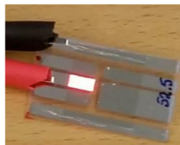
Figure 11. OLEDs printed by VTT. (Credits to IN-LIGHT Project [13])
