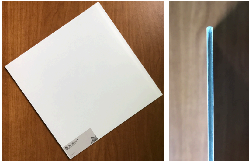
Figure 10. Top layer in glass with white ceramic enamel
