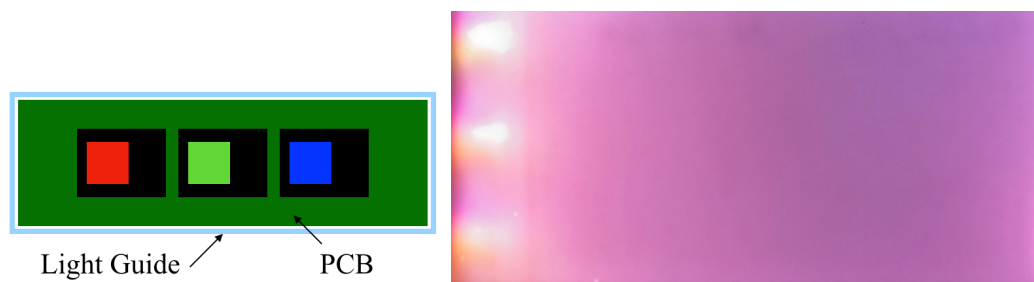
Figure 27. In line placement of the RGB LEDs triplet and the resulting separation of primary components over the tile
