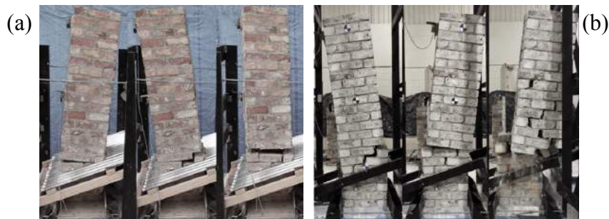
Figure 7.4 Frames of the dynamic response of URM chimneys (taken from Giaretton et al. [6]): progression of rocking for C1(A) (a) and rocking associated with disintegration of mortar for C2(B) (b).
