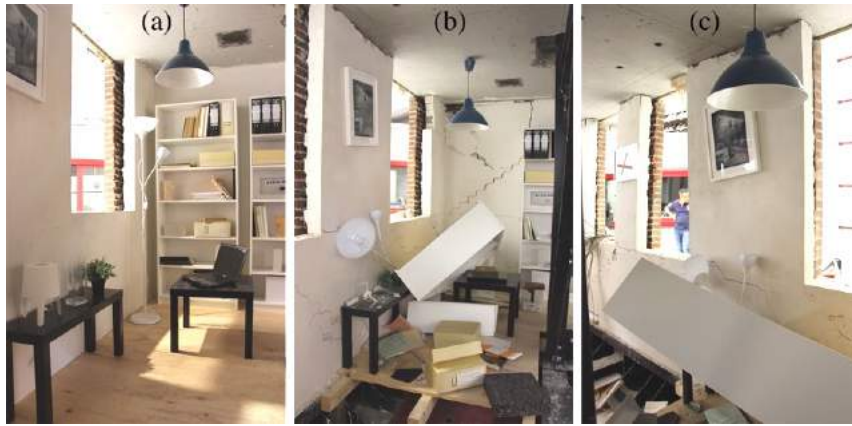
Figure 3.12 Pictures of the building furniture: (a) before testing, (b, c) after FEQ2-300% test.
