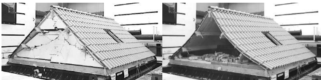
Figure 6.4 Frames of the video of LNEC-2 roof taken during F2EQ2-600% test showing the collapse of the gable wall and the final deformation of the timber diaphragm [7].
