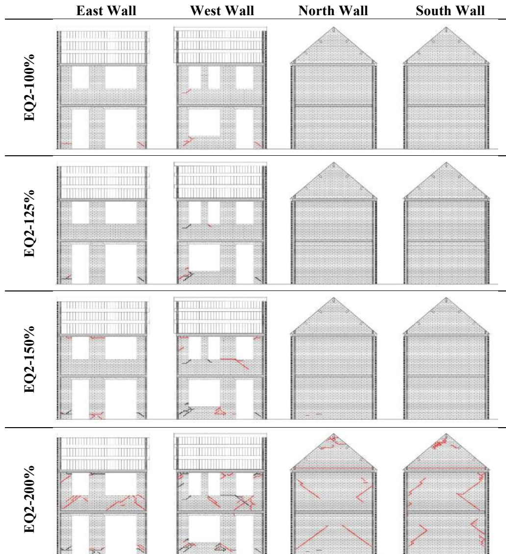
Figure 2.11 Crack pattern evolution of the inner CS walls
