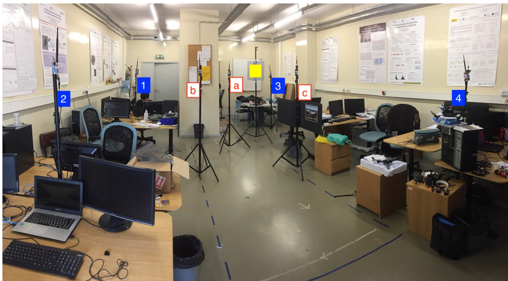
(b) Deployment of 4 anchors (blue) and 3 tags (red) with an artificial obstacle (yellow).
