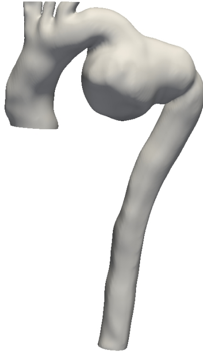
Figure 4.14 Original branched patient-specific surface used to test the "local refinement" capability addition to the "conduction-based" method, after clipping and capping operations performed using the VTK-based Python code described in Section 4.2.
