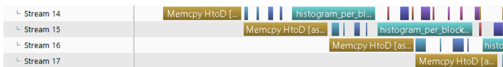
Figure 3.10: NVIDIA Visual Profiler output. Brown boxes represent memory transfers from host to device, while the other boxes concern different kernel executions.
