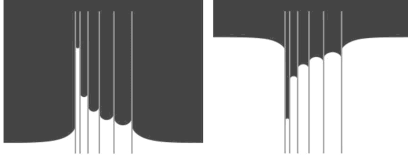
Figure 2.21: Simulation of capillary rise and depression in pipes of different size, performed with a free surface lattice Boltzmann-method [Attar and Körner, 2009].
