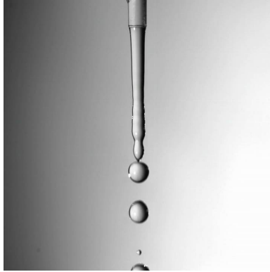
Figure 2.20: Example of Rayleigh instability on fluid water cylinder parallel to gravity direction.
