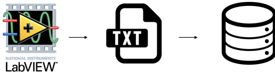
Figure D.4: Filling schema strategy for Italian sites. Output files from steering programs (LabView) are converted in a suitable form by automatic script and uploaded to the database
