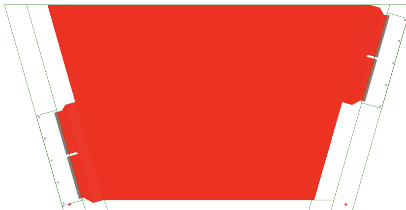
Figure 3.10: Layout of a readout PCB, with indication of the location of the contacts for the front-end electronic boards
