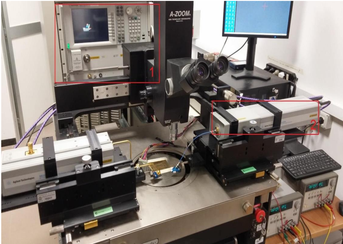
Figure 5.3: small signal measurements setup, 1. VNA, 2. Mixer.
