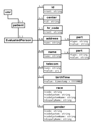
Figure 5.3: Diagram of the XML tags for the patient's demographics.
