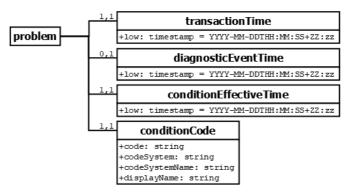
Figure 5.7: Diagram of the XML problem tag.
