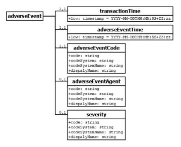
Figure 5.6: Diagram of the XML adverseEvent tag.
