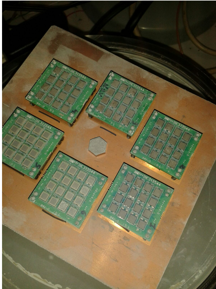
Figure 4.2: Photo of the SiPMs array after the TPB evaporation session on the active surfaces.
