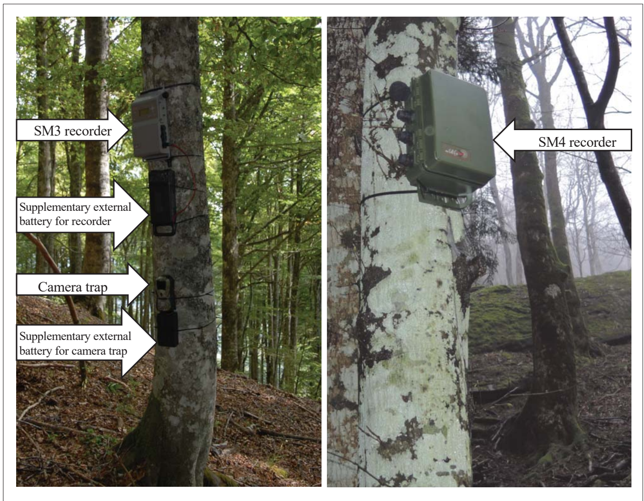
Figure 4.3 On-site positioning of remote autonomous Wildlife Acoustics recorders (model SM3 on the left and SM4 on the right, respectively) inside Sasso Fratino Integral Nature Reserve. In the left photo, the acoustic sampling has been completed with the placement of a camera trap and external batteries for both the recorder and the camera trap in order to prolong the recording time.
