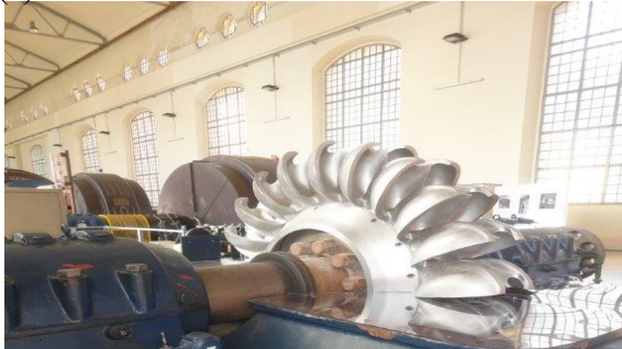
Figure 3.1.6: (a) : The building of an hydroelectric power plant in the Alps, Italy. (b) : A modern computer-based control and monitor scheme of hydroelectric power plant. (c) : A Pelton wheel. (d) : Numerical data of a Pelton wheel. [Credits: Gianmario Rinaldi].
