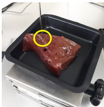
Figure 1.14. Photo of a liver sample during dielectric measurement with the probe inserted in the barely visible slit.
