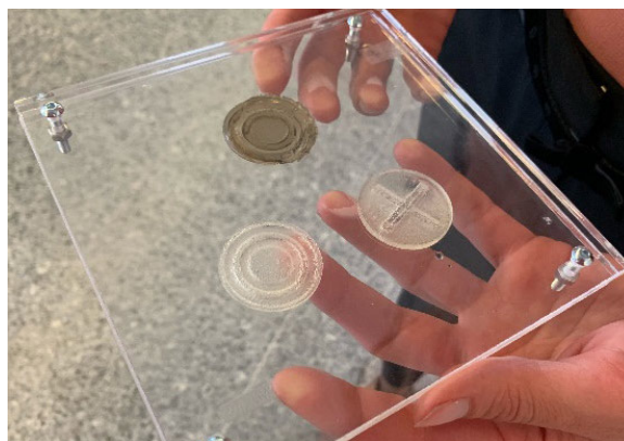
Figure 1.2: Artificial human disposal patches providing fast relief to civilians or military personnel injured by chemical agents [17].
