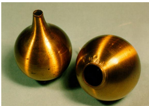
Figure 5.1: Close-up view of two small Helmholtz resonators [2].
