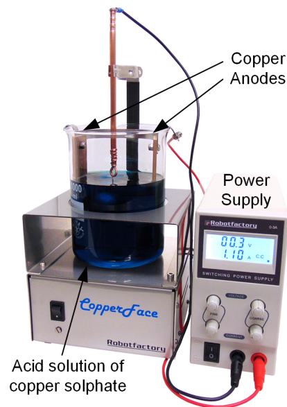
Figure 5.9: The galvanic machine used to metalize the sensor [7].
