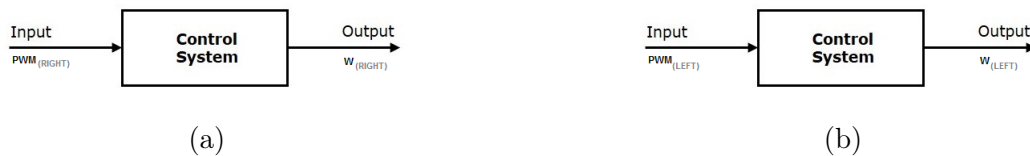
Figure 4.52: Control System represented by SISO model, for right (a) and left (b) motor
