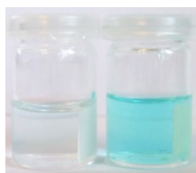
Figure 3. Photographs of a 1.0 x 2.0 cm silica dipstick immersed in a 2 ml of PBS (0.01 mM, pH 7.0) and with 0.18 ml of SQ (acetonitrile, 1.0 x 10 -4 M). The right-handed stick was previously immersed in formaldehyde (1 mM) for 5 min, whereas the left-handed foil was directly dipped into PBS-SQ solution.
