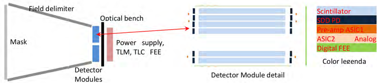
Figure 35: XGIS unit main building blocks.
