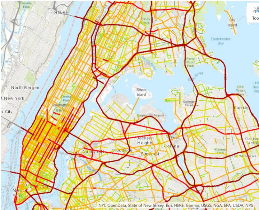
Figure 7.4: a map representing the average daily traffic in New York. It can be noticed that the main highways, the bridges/tunnels and the southern half of Manhattan are the most occupied areas.
