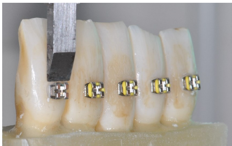
Figure 25. Shear bond strength test. Bracket base was set parallel to shearing force.
