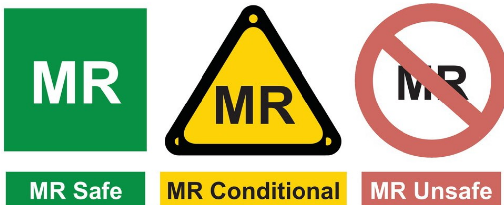
Figure 5 ASTM symbols on RM safety: the first square (green) corresponds to “MRI safe”; the triangle (yellow) corresponds to “MRI conditional”; the circle (red) corresponds to “MR unsafe”.
