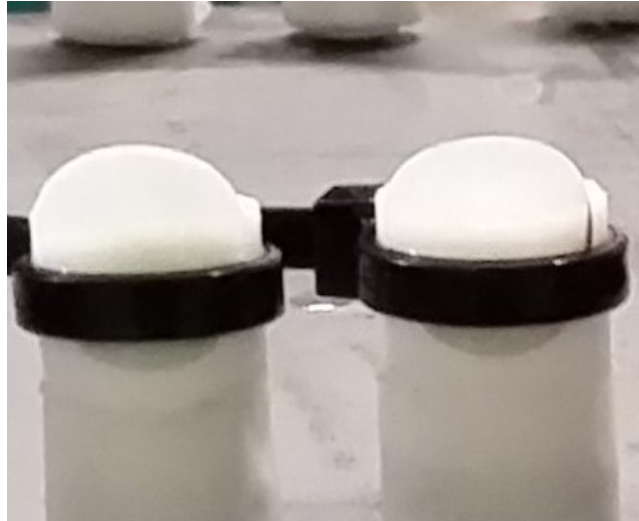
Figure 10. Hoof membranes mounted on PTFE custom made supports.
