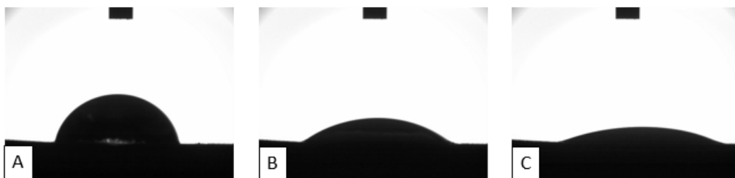
Figure 47. Membrane 4.10.9 (placebo group) before the beginning of the study (t0). A: 0s after drop deposition; B: 30s; C: 60s
