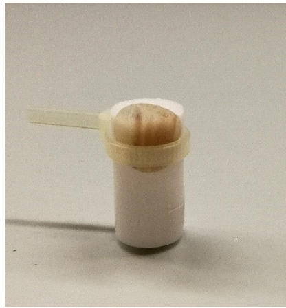
Figure 16. A membrane in the thickness range of 300-400 \mu\text{m} mounted on a PTFE custom made support
