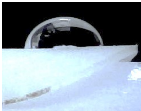
Figure 98. Digital image of the interface phenomenon between the water drop and the membrane
