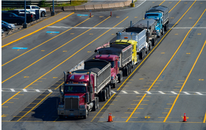
Figure 1.4: Heavy-duty vehicles driving close behind each other, forming a platoon, experience a reduced aerodynamic drag, and a consequent fuel consumption reduction. (Photo from Pinterest)
