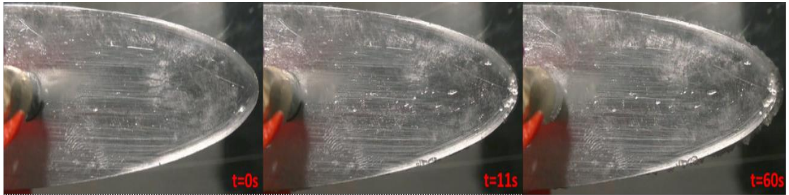
Figure 55. Icing wind tunnel test of SiO 2 FSO10 sample in glaze ice conditions.
