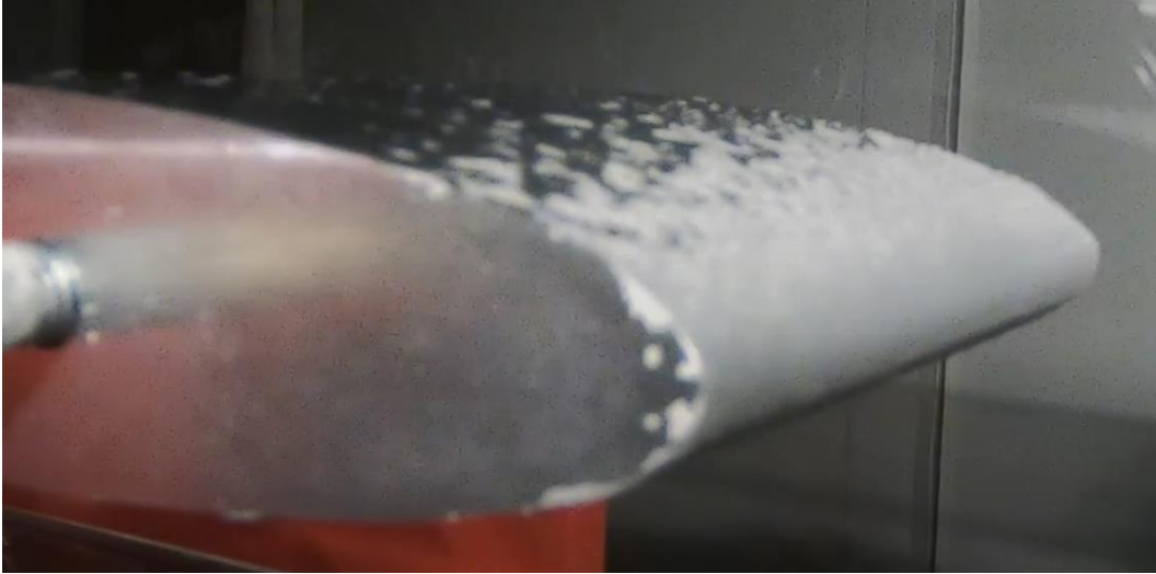
Figure 58. SiO 2 FSO10 sample after icing wing tunnel test in rime ice conditions.
