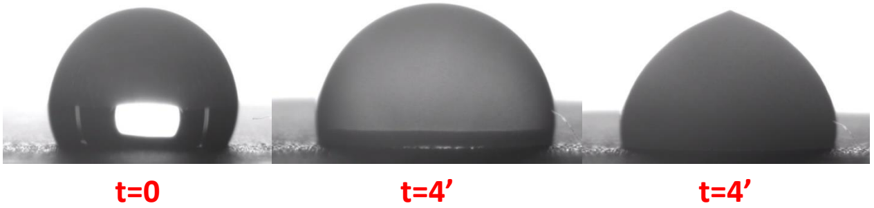
Figure 37. Drop freezing process on LF surface
