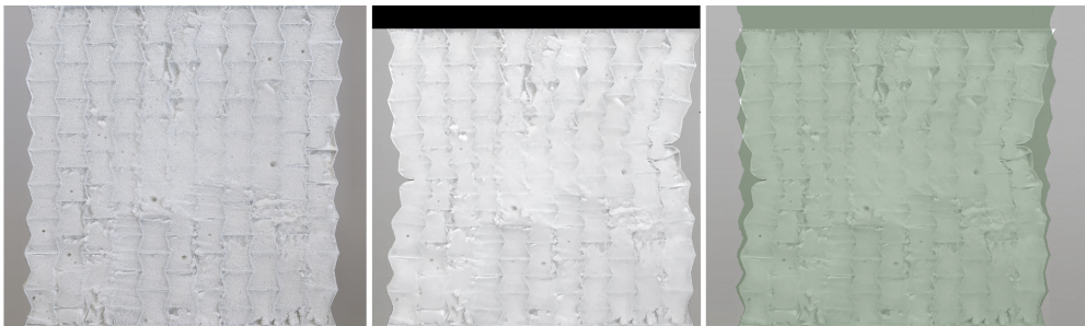
FIGURE 6.28: Specimen-1 tested in compression: undeformed configuration (left), deformed configuration at the end of the loading process (middle), comparison between the undeformed configuration, in green, and the deformed configuration at the end of the loading process (right).
