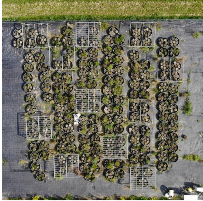
Figure S1. Aerial view of the mesocosm experiment, showing the large 260-L pools with the smaller 20-L pots within. The white grids are the partial rainout shelters to reduce natural precipitation by 30% for the chronic drought treatment. Note that the experiment described here included 40 grassland community pots and 10 bare soil pots in 49 different pools (i.e. not all pools and pots in the picture were part of the experiment described here). Picture: V. Ferenc (June 2018).
